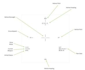
Figure 2. Heads-up display with labeled information elements. Can be customized by the Soldier.
